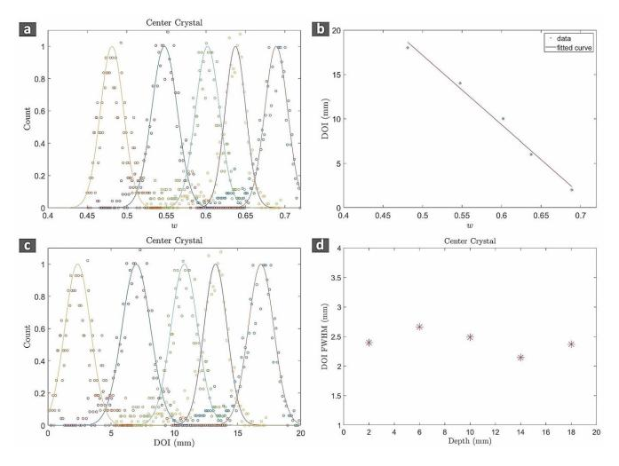
**SUPPLEMENTAL FIGURE 1.** Conversion from DOI-specific *w* histograms to DOI histograms showing the DOI resolution of a single crystal at each depth. (A) Histograms of the DOI-estimation parameter *w* acquired at 2, 6, 10, 14 and 18 mm. (B) Fit between *w* and DOI via linear regression. (C) DOI histograms generated by taking the *w* histograms in (A) and multiplying by the slope of the linear fit in (B). (D) DOI resolution at each acquired depth based on the width of the Gaussians in (C).
