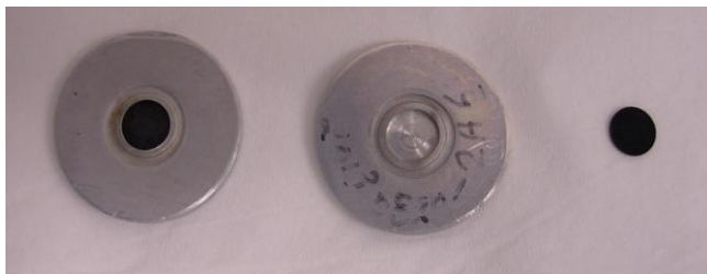
SUPPLEMENTAL FIGURE 2. Undissolved part of ^{100}\text{Mo} pellet detached from aluminium support after decay of irradiated target.
