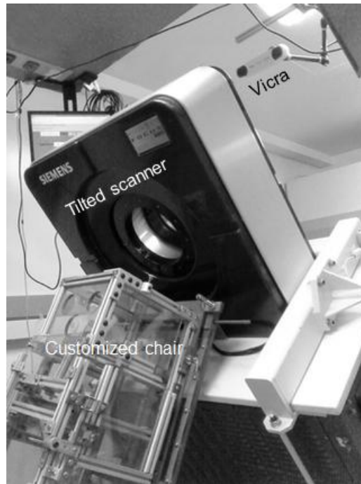
Supplemental Figure 4. MicroPET scanner FOCUS-220 raised and tilted forward \sim 45^\circ with a lifter-tilter. The Vicra camera was hung on the ceiling and positioned towards the bore of the scanner.
