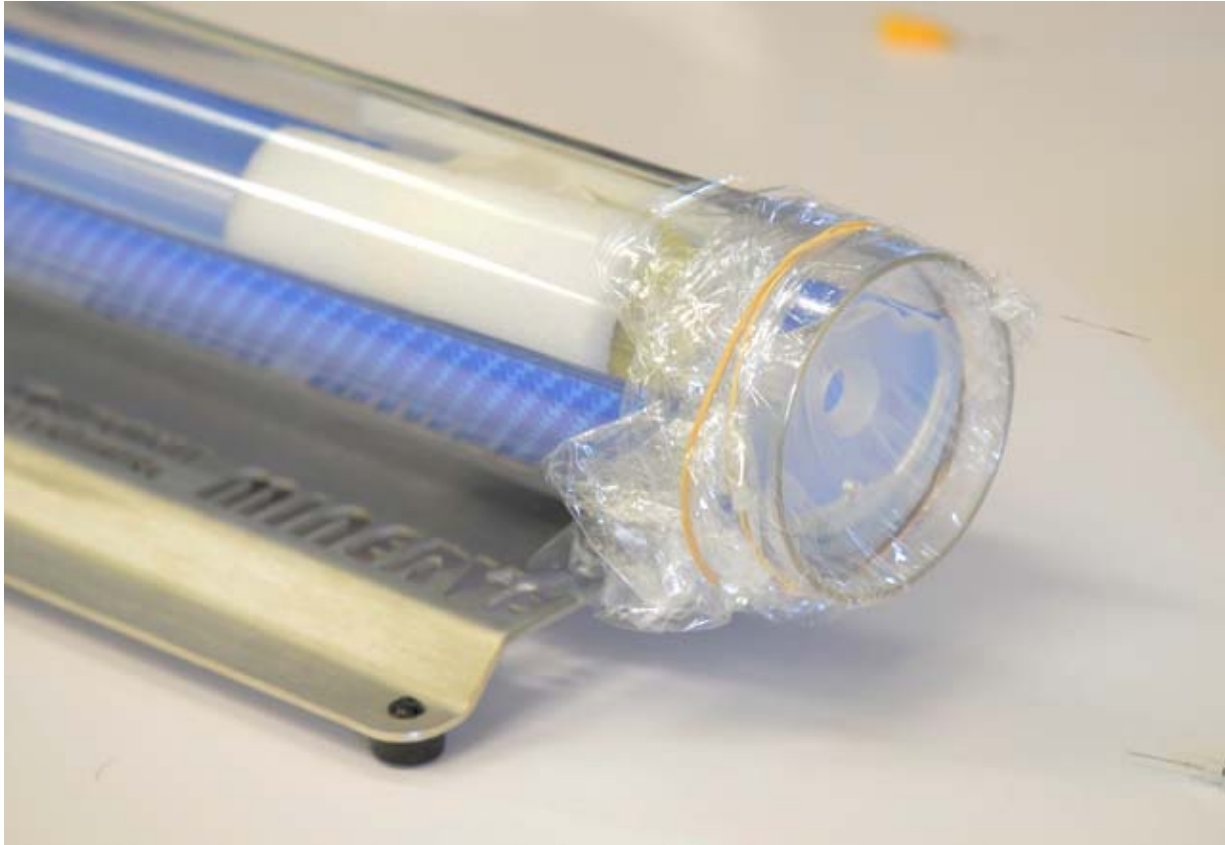
Supplemental Figure 3: Photograph showing the catheterized egg in the Minerve anesthesia cell, held in position using protective foam packaging. The catheter was routed through the open end of the cell cover and an airtight seal fashioned using plastic film.
