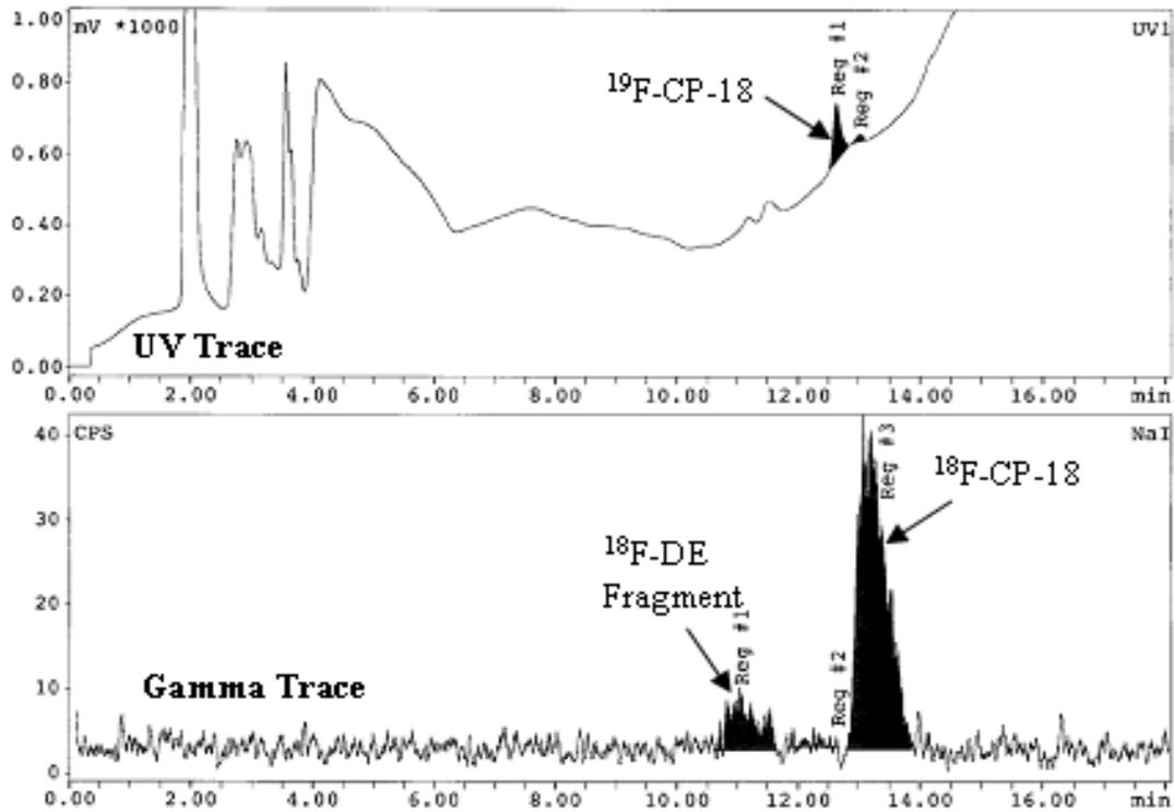
Supplemental Figure 1. A representative radioHPLC analysis of a human plasma sample at 35 minutes post-injection. The UV signal of non-radioactive CP18 (upper trace) overlaps with the predominant radioactive signal in the gamma trace (lower trace), which is un-metabolized  $^{18}\text{F}$ -CP18. The plasma metabolite observed in the gamma trace is tentatively assigned as the fragment cleaved between “DE” and “VD”.
