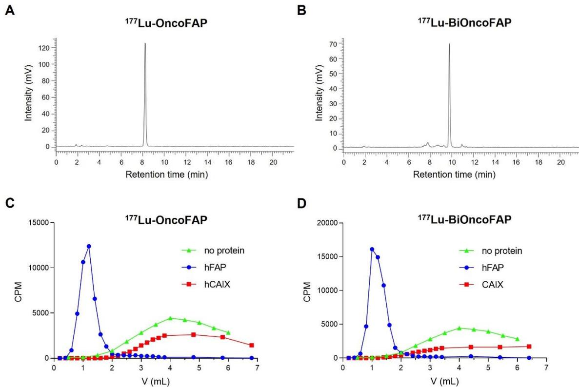
Supplemental Figure 1. Quality control of radiosynthesis. Radio-HPLC of  $^{177}\text{Lu-OncoFAP}$  (A) and  $^{177}\text{Lu-BiOncoFAP}$  (B); PD-10 experiments of  $^{177}\text{Lu-OncoFAP}$  (C) and  $^{177}\text{Lu-BiOncoFAP}$  (D) incubated with hFAP, using no protein or irrelevant protein (hCAIX) as a negative control.
