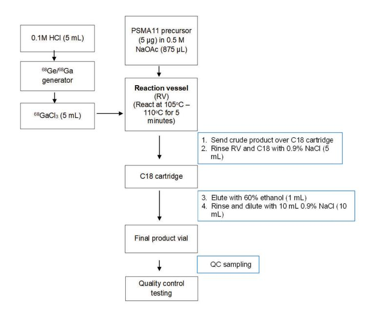
Figure 4: <sup>68</sup>Ga-PSMA-11 Production Method (Generator-based) from UCSF NDA 212643
