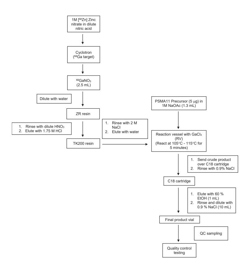
Figure 3: <sup>68</sup>Ga-PSMA-11 Production Method (Cyclotron-based) from UCSF NDA 212643
