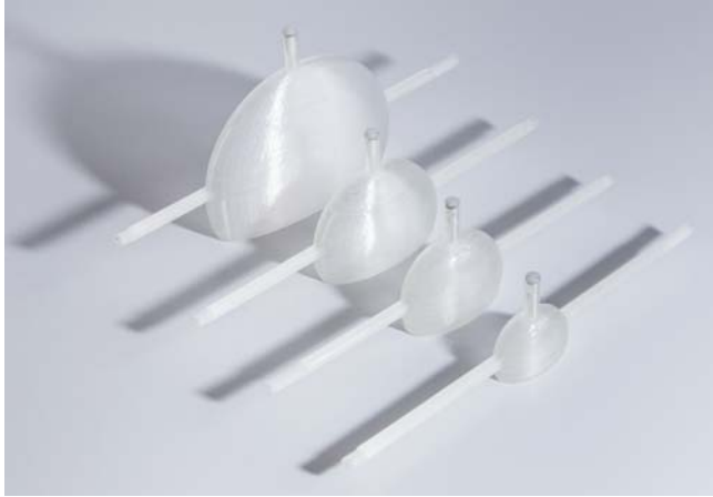
Figure 3: Manufactured set of kidney phantoms. Smallest to largest: Newborn, 1-year-old, 5-year-old, adult.
