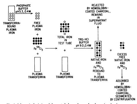
Fig. 1. Schematic depiction of the coated charcoal assay for plasma iron level.
