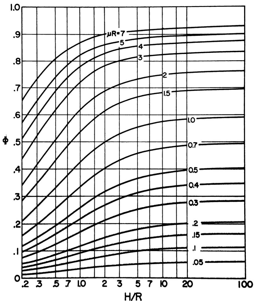
Fig. 1. Absorption fraction as a function of  $\mu R$  and  $H/R$  ( $\mu$  = absorption coefficient,  $R$  = cylinder radius,  $H$  = cylinder height).
