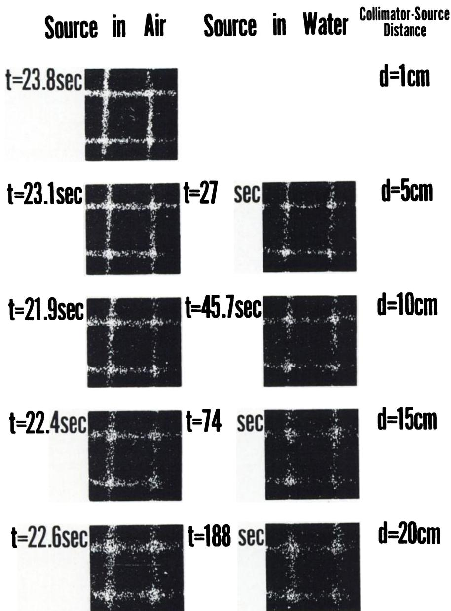
Fig. 5. Scintiphotos with line-source phantom parallel to collimator face at several distances,  $d$ , in air and in water. For the  $^{203}\text{Hg}$  sources in air, the sensitivity of the scintillation camera is constant for all source-to-collimator distances while the spatial resolution decreases with increasing distance. With the sources in water the exposure time,  $t$ , for a constant number of dots increases rapidly because of  $\gamma$ -ray absorption.
