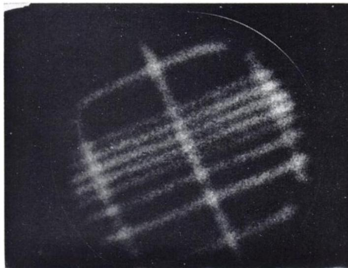
Fig. 2. Scintiphoto of line-source phantom in contact with face of collimator. Using the  $^{203}\text{Hg}$   $\gamma$  rays,  $10^5$  counts were collected. Uniformity of scintillation camera performance for most parts of the field of vision is satisfactory.
