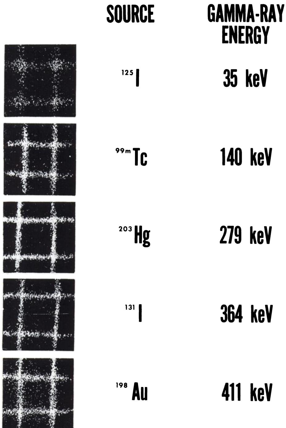
Fig. 3. Dependence of spatial resolution of scintillation camera on  $\gamma$ -ray energy. Line-source phantom with only four sources, 10 cm apart, in contact with 1165-hole collimator, yielded best results with  $^{203}\text{Hg}$  sources.
