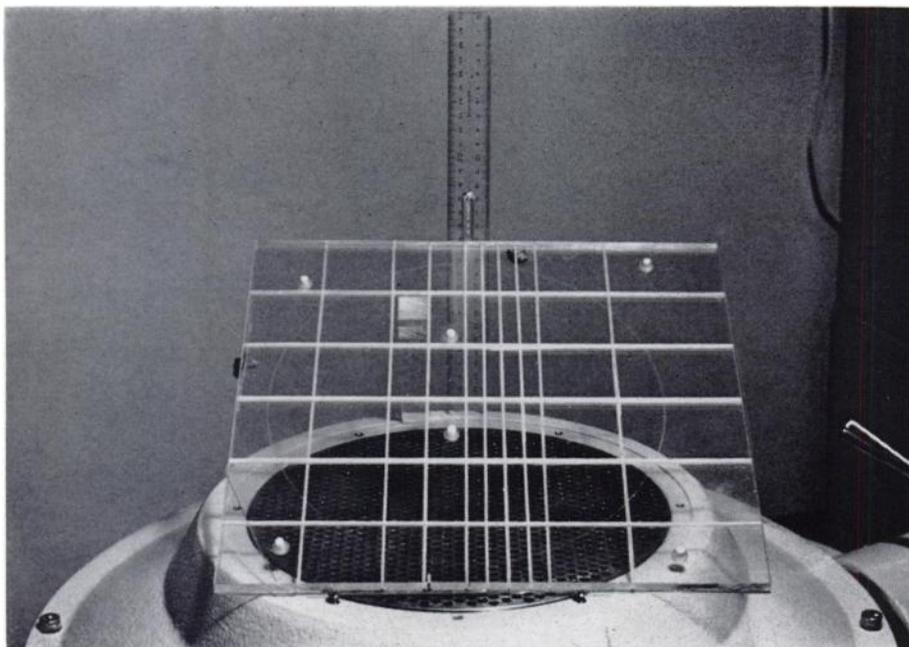
Fig. 1. Line-source phantom in tilted position on top of multichannel collimator of scintillation camera. Thin plastic tubes containing a radioactive solution are placed in grooves of Lucite phantom.
