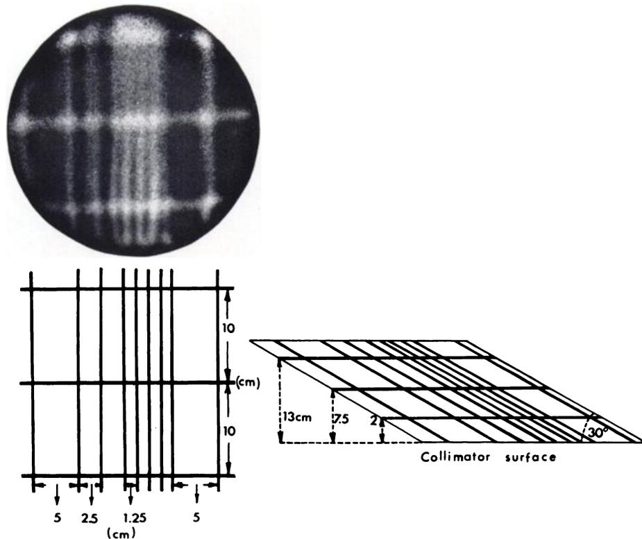
Fig. 4. Test of depth response of scintillation camera with line-source phantom in tilted position as shown in Fig. 1. Results obtained with  $^{203}\text{Hg}$   $\gamma$  rays verify expected camera performance.
