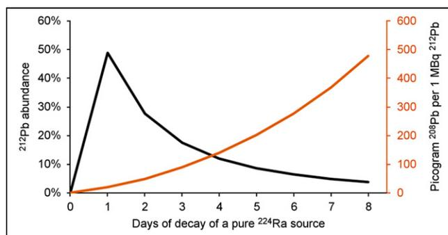
**FIGURE 3.** Relationship between radioactive  $^{212}\text{Pb}$  and stable daughter nuclide  $^{208}\text{Pb}$  as function of time, shown as abundance of  $^{212}\text{Pb}$  relative to total amount of lead (black curve) and mass concentration of  $^{208}\text{Pb}$  per 1 MBq of extracted  $^{212}\text{Pb}$  (red curve), assuming generator yield of 62%.
