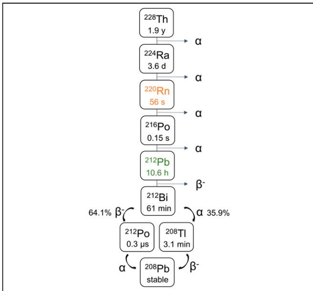
**FIGURE 1.**  $^{228}\text{Th}$  series, with  $^{220}\text{Rn}$  and  $^{212}\text{Pb}$  highlighted.
