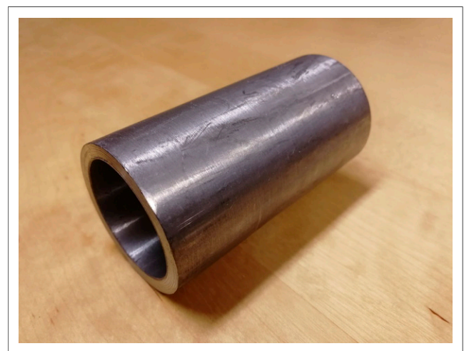
FIGURE 2. Shield of Rose metal for intratherapeutic PET imaging of mice during RNT. Shields used were 2, 3, and 4 mm thick (here shown with 4-mm thickness). All had inner diameter of 35 mm.
