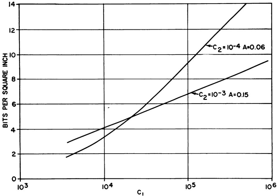
Fig. 3. Information capacity of a Single Bore Collimator as a function of signal for several values of bore area and noise.
