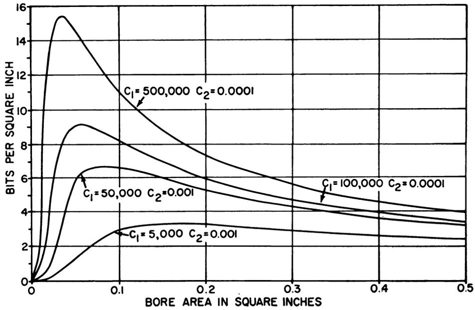
Fig. 1. Information capacity of a Single Bore Collimator as a function of bore area for several values of signal and noise.
