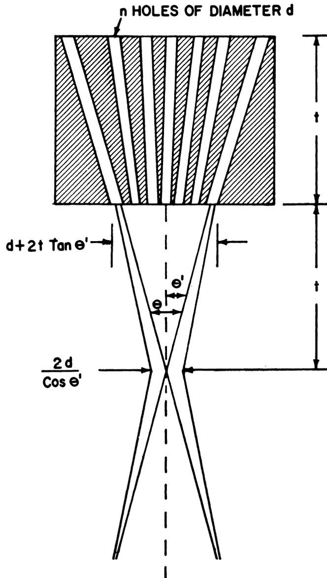
Fig. 7. Geometric relations assumed for Focussing Collimators. The outside lines are the envelope for  $A_s$  as a function of distance from the collimator.
