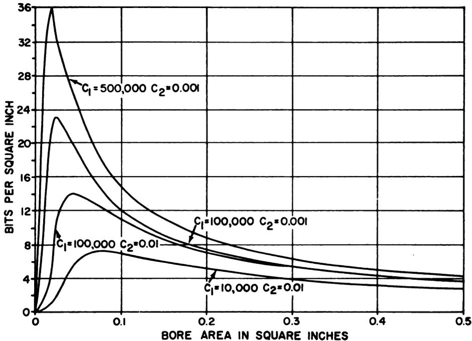
Fig. 8. Information capacity of a Honeycomb Collimator as a function of the bore area of each hole for several values of signal and noise.
