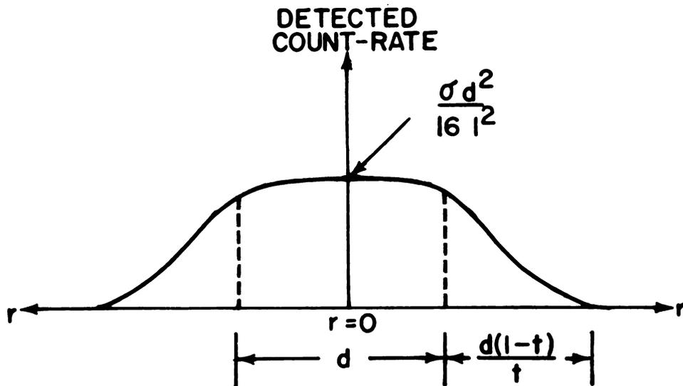
Fig. 5. Approximate count-rate profile for a point source of strength  $\sigma$  moved across the plane shown in Fig. 4.
