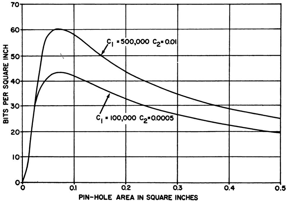
Fig. 10. Information capacity as a function of Pinhole area for several values of signal and noise.
