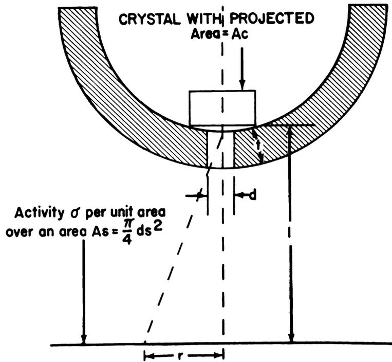
Fig. 4. Geometric relations assumed for a Single Bore Collimator viewing a planar distribution of activity.
