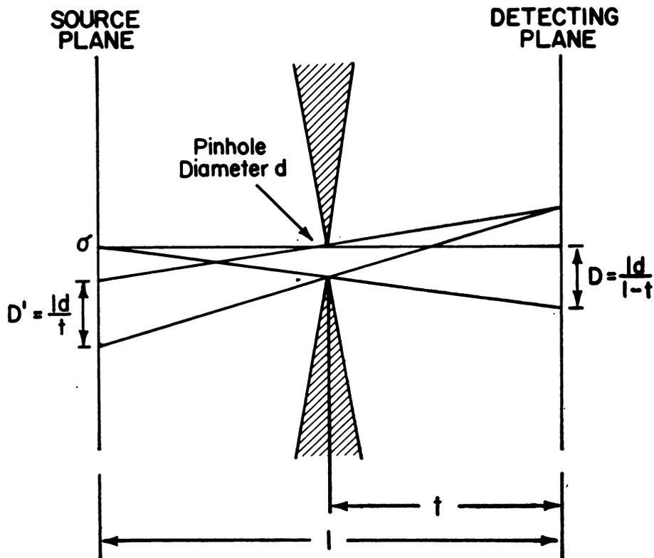
Fig. 9. Geometric relations assumed for a Pinhole camera.
