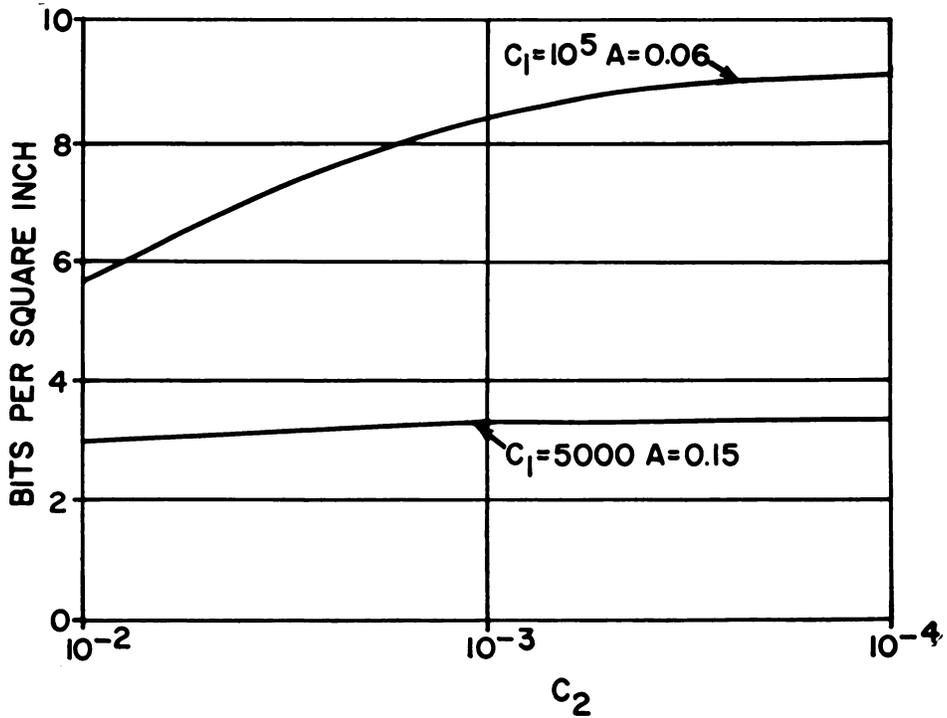
Fig. 2. Information capacity of a Single Bore Collimator as a function of noise for several values of signal and bore area.
