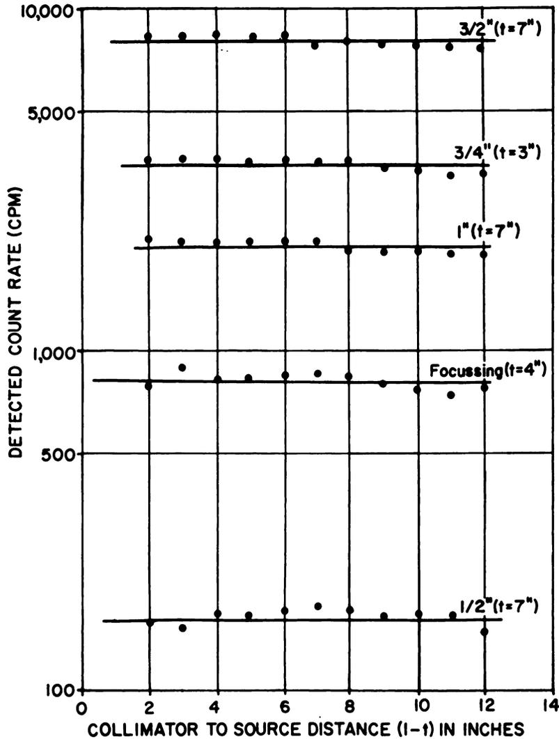
Fig. 6. Observed count-rate as a function of the distance (1 - t) to a planar distribution of activity for various diameter single bore collimators. The source is  $^{131}\text{I}$  with a density of  $1.41 \mu\text{c/sq inch}$ .
