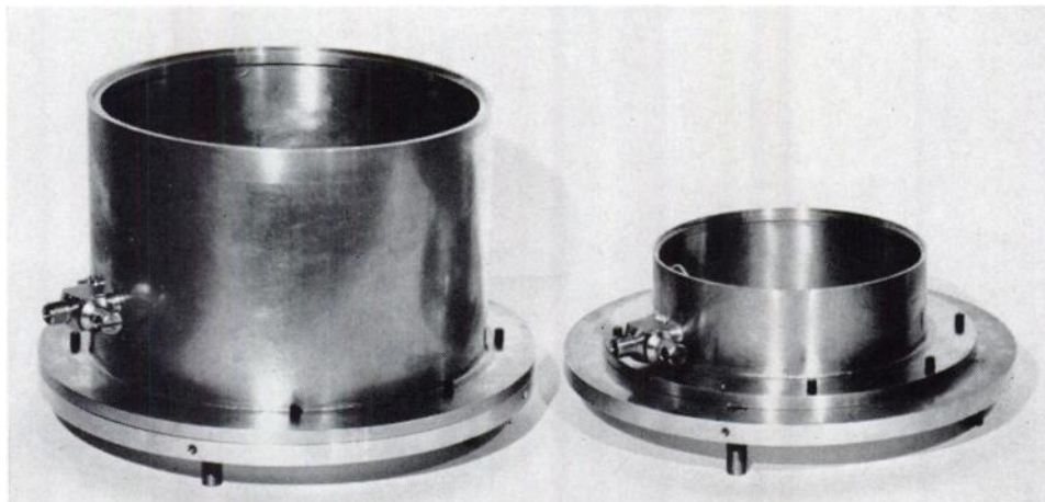
Fig. 6. A 7 inch diameter chamber is shown on the left and the 5 inch "thyroid" chamber on the right. The electrodes have not been sealed into these chambers.
