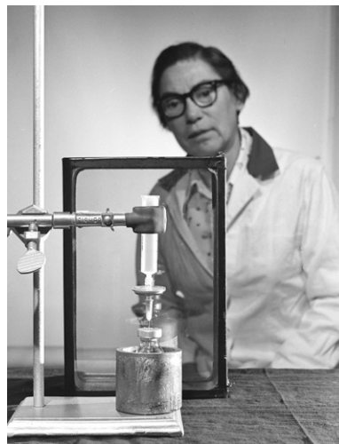
Brookhaven National Laboratory chemist Margaret Greene played a prominent role in development of the original ^{99m}\text{Tc} generator, shown here. From Brookhaven National Laboratory.
