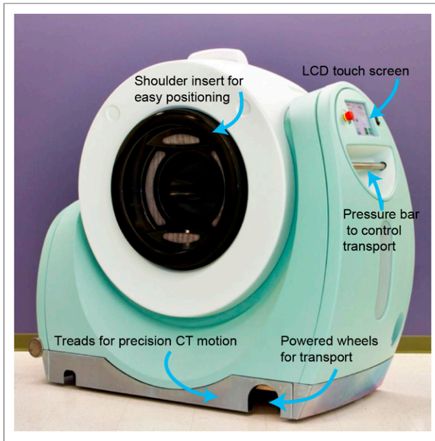
FIGURE 1. NeuroPET/CT scanner with outer components labeled. Treads (behind metal apron) are used for precise scanner motion during CT scans, whereas wheels are used to transport scanner to scan location.
