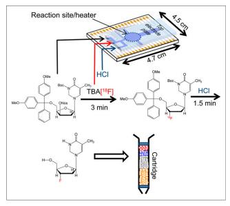
**FIGURE 1.** Overall workflow of radiosynthesis of <sup>18</sup>F-FLT on EWOD chip, followed by cartridge purification to produce injectable dose of <sup>18</sup>F-FLT for mice imaging; synthetic scheme of radiosynthesis of <sup>18</sup>F-FLT using mixture of thexyl alcohol and DMSO in fluorination reaction. Crude <sup>18</sup>F-FLT product was extracted and purified via simple cartridge purification to yield approximately 52 MBq (non-decay-corrected) of <sup>18</sup>F-FLT.
