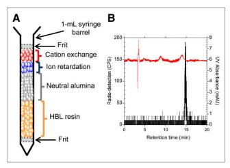
**FIGURE 3.** (A) Custom-made purification cartridge used to purify <sup>18</sup>F-FLT that was synthesized on EWOD chip. (B) High-performance liquid chromatogram of cartridge-purified <sup>18</sup>F-FLT. Red chromatogram represents absorbance in ultraviolet range, and black chromatogram represents radio detection.
