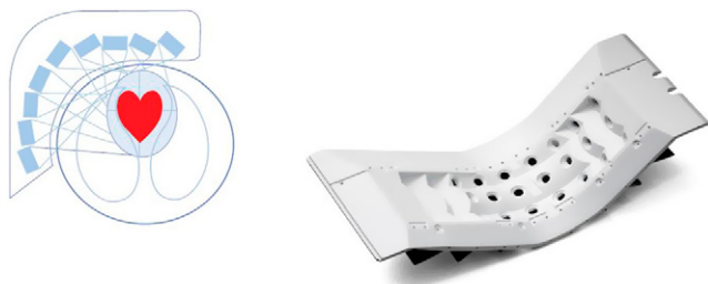
FIGURE 2. GE's design for the 19-pinhole stationary SPECT cardiac camera. Left: schematic drawing of geometry involved whereby each pinhole views the heart from a different angle so as to obtain projections sufficient for 3D reconstruction of radiotracer distribution. Right: actual 19-pinhole array. (Courtesy GE Healthcare).
