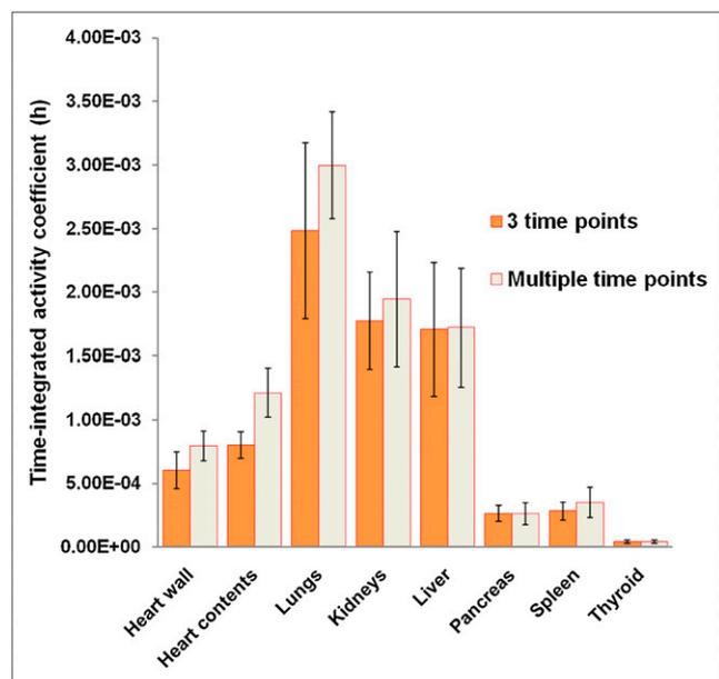
**FIGURE 2.** Comparison of mean TIAC (h) calculation at rest based on 3-time-point whole-body PET (current study) and multibed multiple-time-point PET (previous study (2)) for selected source organs.
