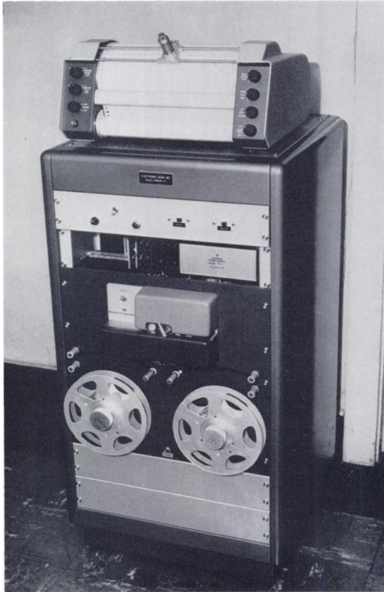
Fig. 7. The paper tape instructions control the plotter in accordance with the computer analysis.
