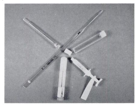
Fig. 1. Materials used in performance of the resin sponge I<sup>131</sup> T3 test: Serum, incubation and counting tube and cap, I<sup>131</sup> T3 capped syringe, resin sponge, 1 ml. pipette and aspirator tip.
