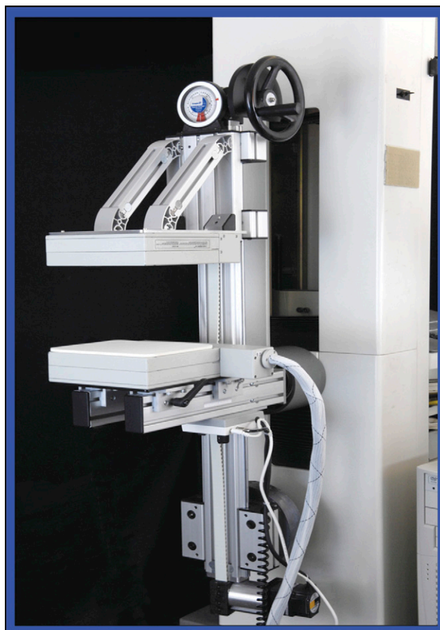
FIGURE 11. Gains in molecular breast imaging are being made with apparatus like this cadmium zinc telluride \gamma camera.
