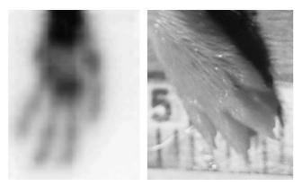
**FIGURE 7.** Projection image of a mouse foot acquired with two 0.5-mm LSO detectors using  $^{18}\mathrm{F}^-$  as radiotracer. Photograph of a mouse foot, with a millimeter-scale ruler as reference, is also shown.
