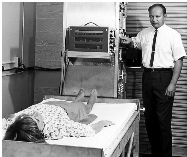
Hal Anger with the Donner whole-body scanner in its 1965 version. In the foreground is the collimator for the 64 scintillation counters. The table moved slowly over the counters in a straight linear motion to obtain a head-to-toe image.
