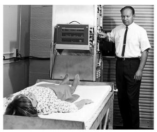
Hal Anger with the Donner whole-body scanner in its 1965 version. In the foreground is the collimator for the 64 scintillation counters. The table moved slowly over the counters in a straight linear motion to obtain a head-to-toe image.
