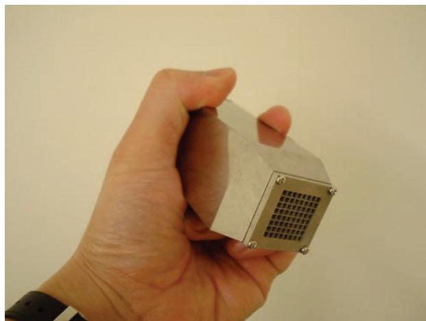
FIGURE 25. Hand-held positron imaging detector with background rejection capability for high-resolution, real-time imaging.
