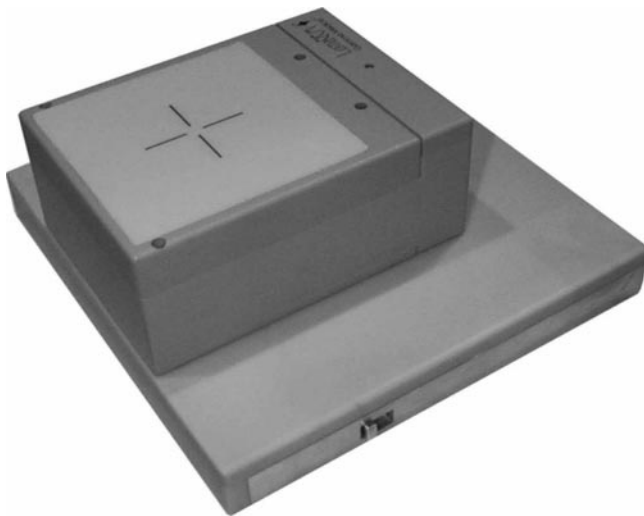
FIGURE 1. Dedicated breast camera attached to an adapter that allows the unit to be mounted on most mammography units.
