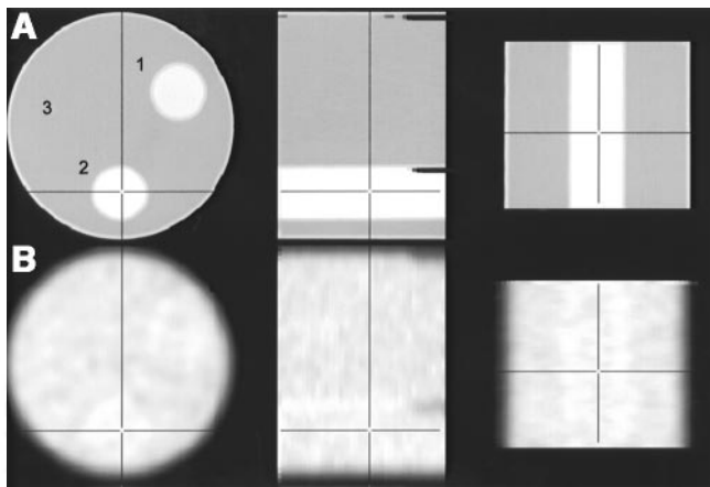
FIGURE 2. Attenuation images of NEMA phantom containing 2 cylindric acrylic inserts with oral CT contrast agent in clinical concentrations. Row A shows orthogonal CT sections (140 kV, 160 mA); row B shows matched PET transmission images acquired with ^{68}\text{Ge} rods in 30 min. Slight attenuation increase originating from insert walls is notable in transmission images. 1 = Micropaque Scanner; 2 = Gastrografin; 3 = water.
