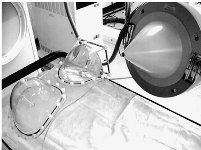
FIGURE 5. Phantom experiment setup includes anthropomorphic phantom and portable gamma camera with pinhole collimator aimed at lateral side of breast. Seven projections were taken of breast at different angles. These projections were then reconstructed using ETACT software to create slices through breast.
