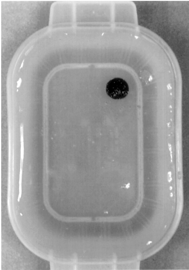
FIGURE 2. Gelatin compressed-breast phantom containing 10-mm-diameter simulated lesion.
