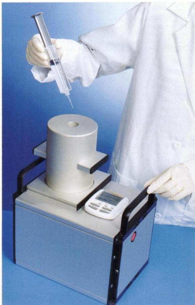
**FIGURE 3.** Clinical  $^{62}\text{Zn}/^{62}\text{Cu}$  generator with collection syringe ready for insertion.
