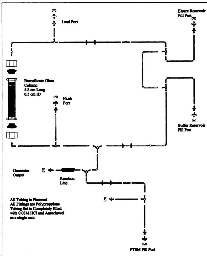
FIGURE 1.  $^{62}\text{Zn}/^{62}\text{Cu}$  generator tubing set assembled for autoclaving.
