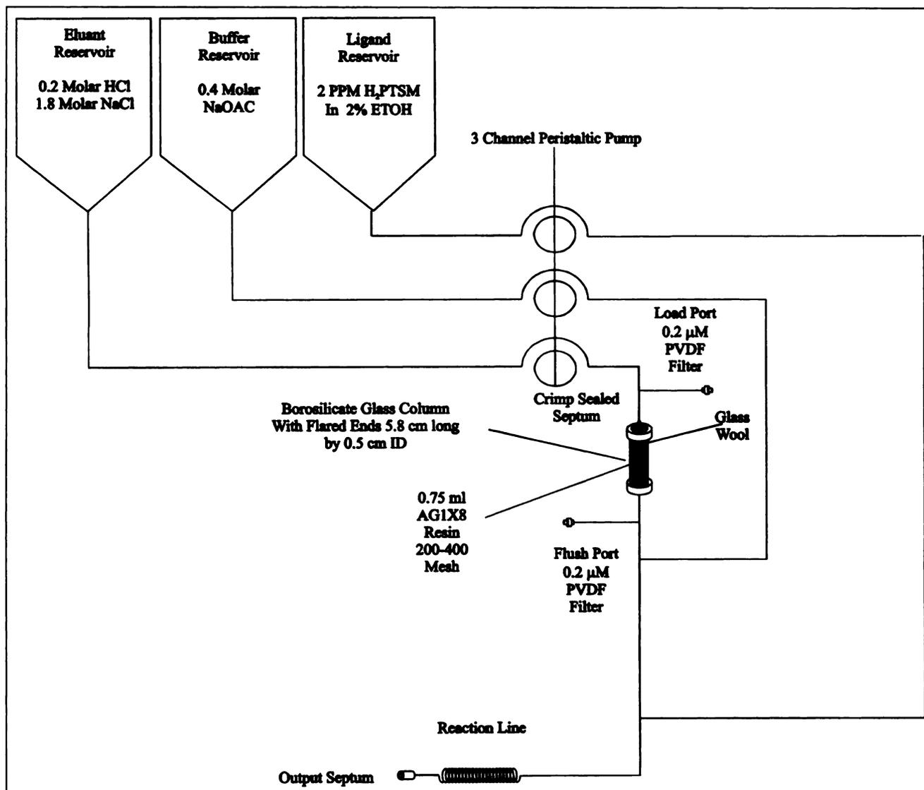
FIGURE 2.  $^{62}\text{Zn}/^{62}\text{Cu}$  generator schematic.
