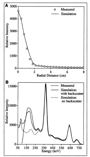
FIGURE 1. Measured and simulated radial PSFs (A) and energy spectra (B) for point source in air.
