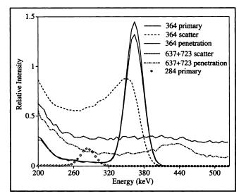
**FIGURE 6.** Spectra of 284-, 364-, and 637 + 723-keV  $\gamma$ -rays separated according to type of interaction for ROI indicated in Figure 5C.
