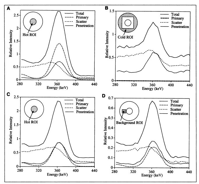
FIGURE 5. Total, primary, scatter, and penetration components of energy spectrum corresponding to ROIs indicated by shaded regions in inset. (A) Hot sphere ROI for phantom with no background activity. (B) Cold ROI for phantom with no background activity. (C) Hot sphere ROI for phantom with background activity. (D) Background ROI for phantom with background activity.
