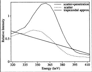
**FIGURE 7.** Scatter spectrum, scatter and penetration spectrum, and trapezoid approximation (approx) in photopeak window for ROI indicated in Figure 5A.
