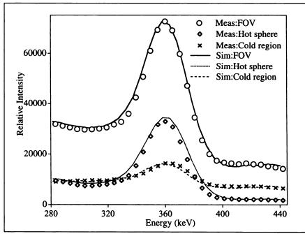
FIGURE 2. Measured (Meas) and simulated (Sim) FOV and ROI energy spectra for hot sphere phantom with no background activity.
