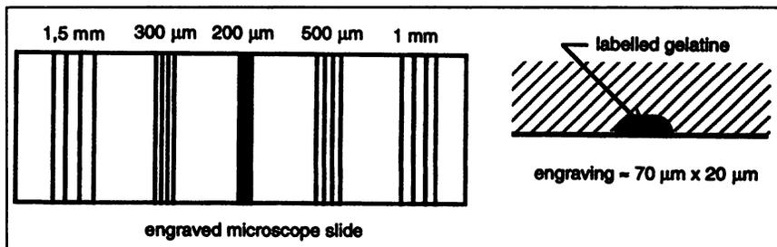
**FIGURE 6.** Special sample for resolution measurements.
