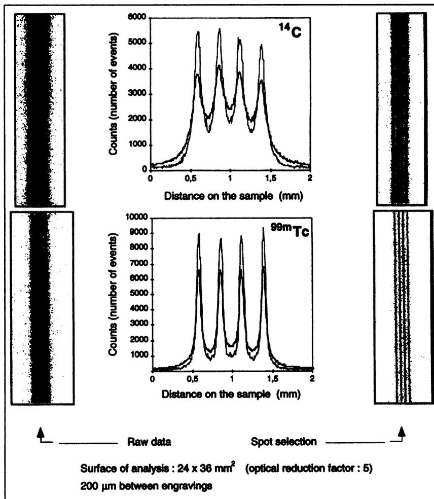
**FIGURE 7.** Spatial resolution measurements for  $^{14}\text{C}$  and  $^{99m}\text{Tc}$ . Comparison of results obtained from raw data and after spot selection.
