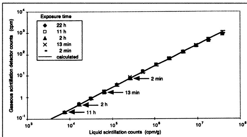
FIGURE 5. Linearity measurements with  $^3\text{H}$ ; limit of sensitivity after indicated exposure time.
