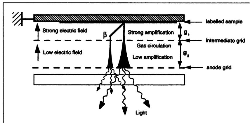
**FIGURE 3.** High amplification mode in two-stage structure.
