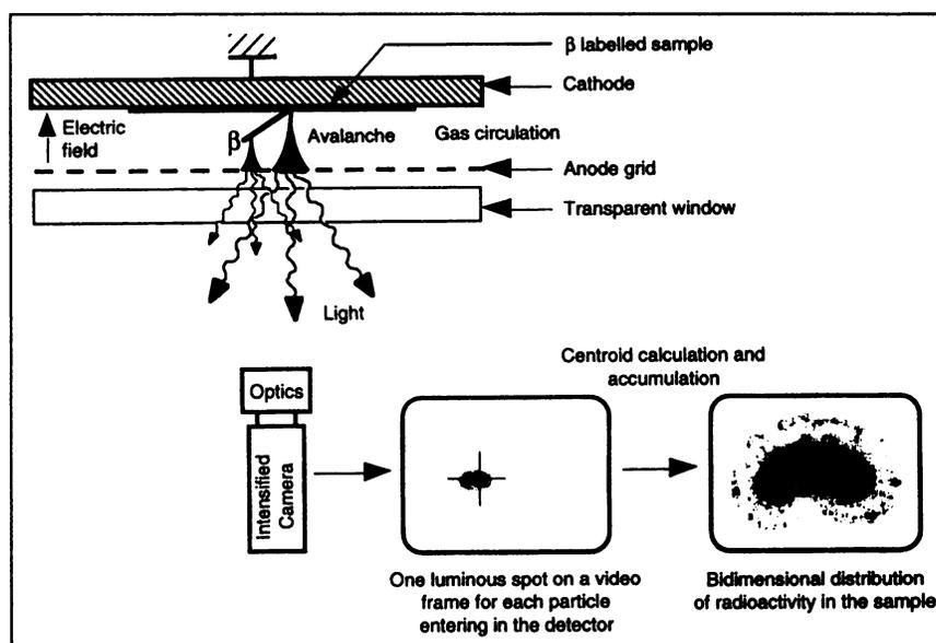
**FIGURE 2.** General principle of detection.
