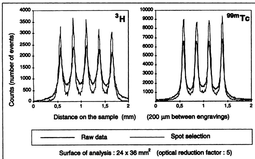
FIGURE 8. Spatial resolution measurements; comparison of results for  $^3\text{H}$  and  $^{99\text{m}}\text{Tc}$ .
