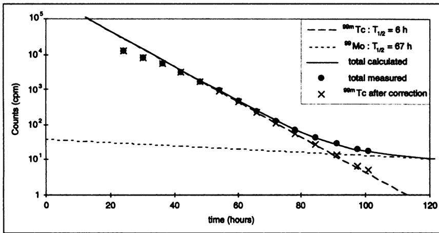
FIGURE 4. Linearity measurements using short half-life of  $^{99m}\text{Tc}$ .
