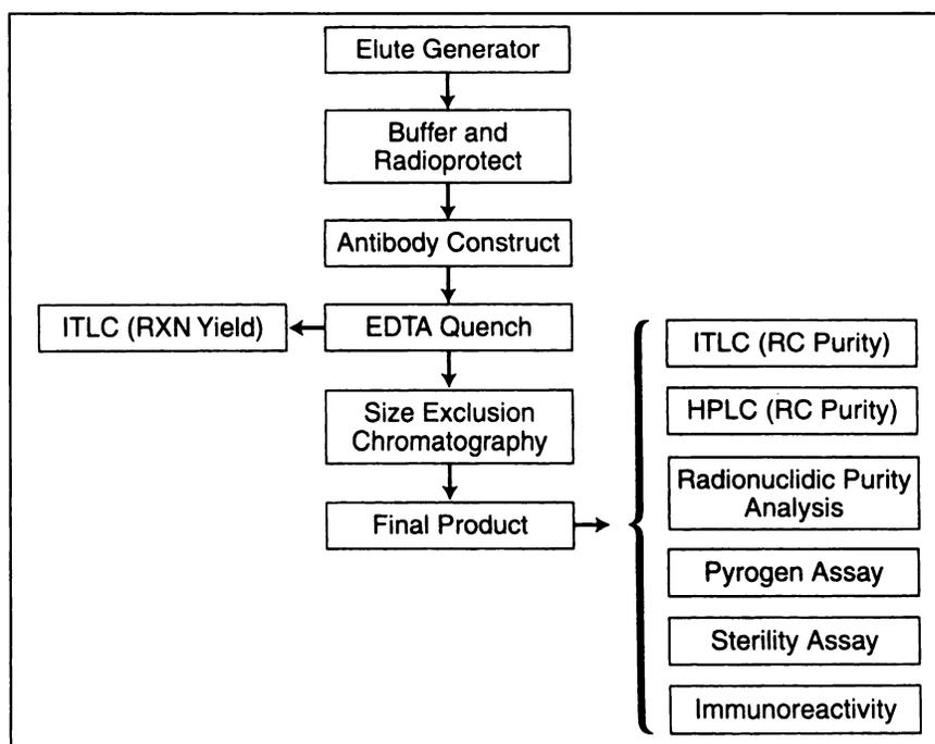
**FIGURE 2.** Flow diagram for  $^{213}\text{Bi}$  radiolabeling of the antibody construct and quality control process. ITLC = instant thin-layer chromatography; RXN = reaction; EDTA = ethylenediaminetetraacetic acid; RC = radiochemical; HPLC = high-performance liquid chromatography.
