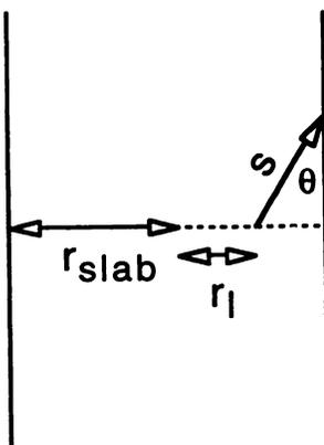
**FIGURE 4.** Slab geometry of marrow cavities in ribs, clavicle, sternum and pelvis. The point of emission of a beta particle was located at a distance  $r_1$  from the slab center. The emission angle was  $\theta$ . The distance from the emission point to the geometrical surface was  $s$ . The half-thickness of the slab was  $r_{\text{slab}}$ .
