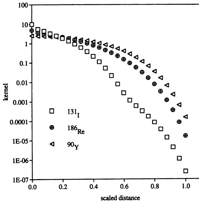
**FIGURE 1.** Dose point kernels ( $10$ ) of <sup>131</sup>I, <sup>186</sup>Re and <sup>90</sup>Y radionuclides are plotted as a function of the scaled distance. The integral of the kernels over the scaled distance is normalized to unity. Actual distances are obtained by multiplying the scaled distances by the CSDA appropriate for the radionuclide.
