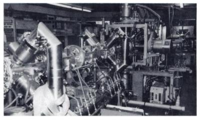
fications are completed over the next few months, LINAC will provide 1 mA of current at 70 MeV of energy. In comparison to U.S.-based commercial cyclotrons, LINAC will generate four to five times the beam intensity and more than two times the energy levels.
