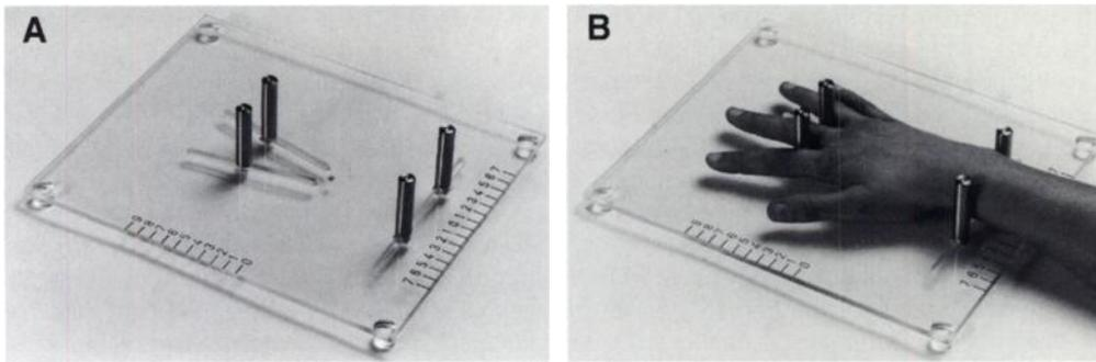
**FIGURE 1.** (A) The hand-fix device for obtaining the radiographs with three lead markers. (B) Positioning the wrist in the hand fix.
