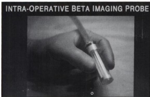
**Figure 9.** Unlike simpler nonimaging probes, the beta detecting imaging probe is not as dependent on the surgeon to direct it.
