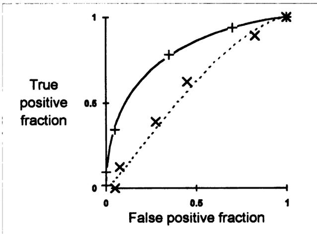
**FIGURE 4.** Comparison between energy-weighted acquisition and discrete energy window of average observer ROC curves for the cold lesion detection task using the Hoffman brain phantom. Fitted energy-weighted acquisition (—); fitted discrete energy window (---); measured energy-weighted acquisition (+); measured discrete energy window (×).
