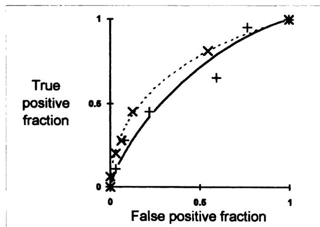
**FIGURE 3.** Energy-weighted acquisition and discrete energy window comparison of average observer ROC curves for the cold lesion on a hot uniform background detection task. Fitted energy-weighted acquisition (—); fitted discrete energy window (---); measured energy-weighted acquisition (+); measured discrete energy window (x).
