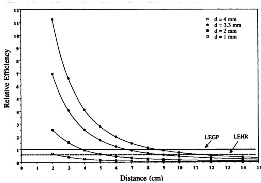
**FIGURE 2.** Relative sensitivity of pinhole collimator plotted as function of distance between collimator and 2.2-cm diameter disk source of  $^{99m}\text{Tc}$  compared with sensitivity of LEHR and LEGP collimators (2). Sensitivity falls rapidly as the distance between collimator aperture and object increases.
