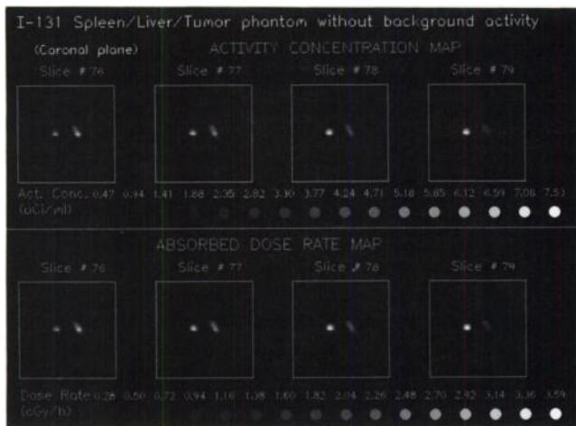
FIGURE 8. Gray-scale images for four coronal sections of Alderson abdominal phantom. Top row shows activity concentration maps, and the bottom row shows absorbed dose rate maps of the corresponding four slices. The round ROI on the left is the tumor, and the oval ROI on the right is the spleen. Gray scales that correlate different shades of gray to the absorbed dose rate and activity concentration are also shown.
