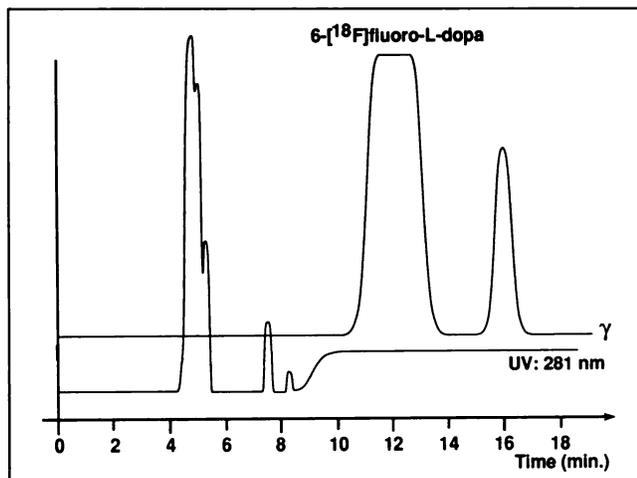
**FIGURE 3.** HPLC purification profile of 6-[<sup>18</sup>F]fluoro-L-dopa. Conditions: Whatman ODS 3 (7 μ) column (9 × 500 mm).
