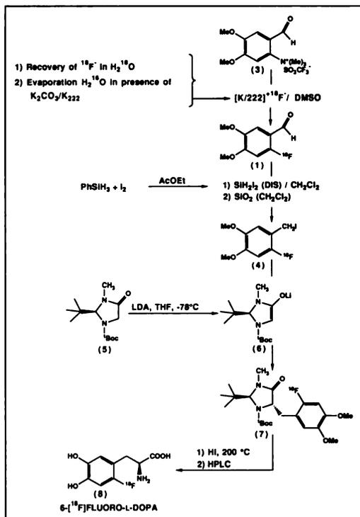
**FIGURE 1.** Radiolabeling of NCA 6-[ $^{18}\text{F}$ ]fluoro-L-dopa starting from its aryltrimethylammonium precursor.
