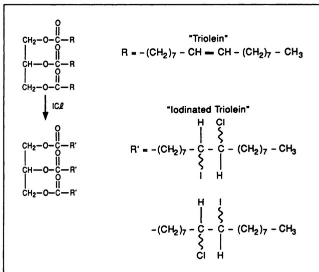
**FIGURE 1.** Possible structures of "radioiodinated triolein" obtained by [<sup>131</sup>I]iodine monochloride (ICl) addition to triolein.
