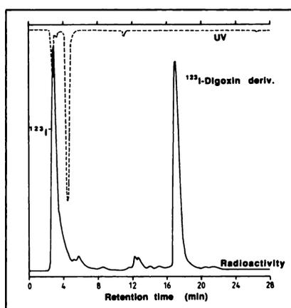
**FIGURE 5.** A typical elution profile of the labeling solution of  $^{123}\text{I}$ -digoxin-iodohistamine(bis(O-carboxymethylloxime)). Elution conditions are described in the text.
