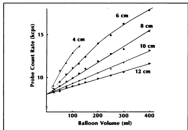
**FIGURE 4.** The relationship between balloon volume and probe count rate in water with background, in various distance from the probe to the center of the balloon. The count rate of the balloon was underestimated when volume was over 200 ml with 6 cm distance from collimator surface to the center of the balloon. However, with 8–12 cm distances there was no underestimation until 400 ml.
