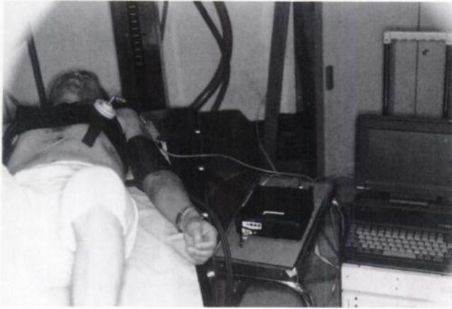
**FIGURE 1.** Continuous ventricular function monitor with CdTe detector. The detector is kept in place by velcro tape attached to an elastic vest-like garment worn by the subject. The portable acquisition unit, battery unit, and personal computer are also shown.
