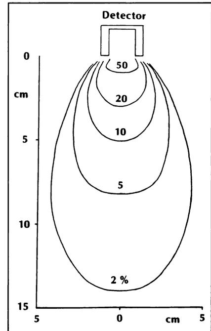
**FIGURE 3.** Isoresponse curves of the cadmium telluride detector in air.
