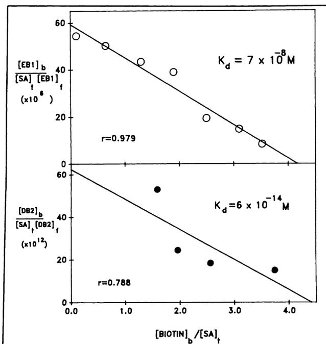
**FIGURE 2.** Scatchard plot for determination of the dissociation constant of EB<sub>1</sub> (top) and DB<sub>2</sub> (bottom). Each point represents an average of duplicate measurements. The dissociation constant is given by the slope of the line.
