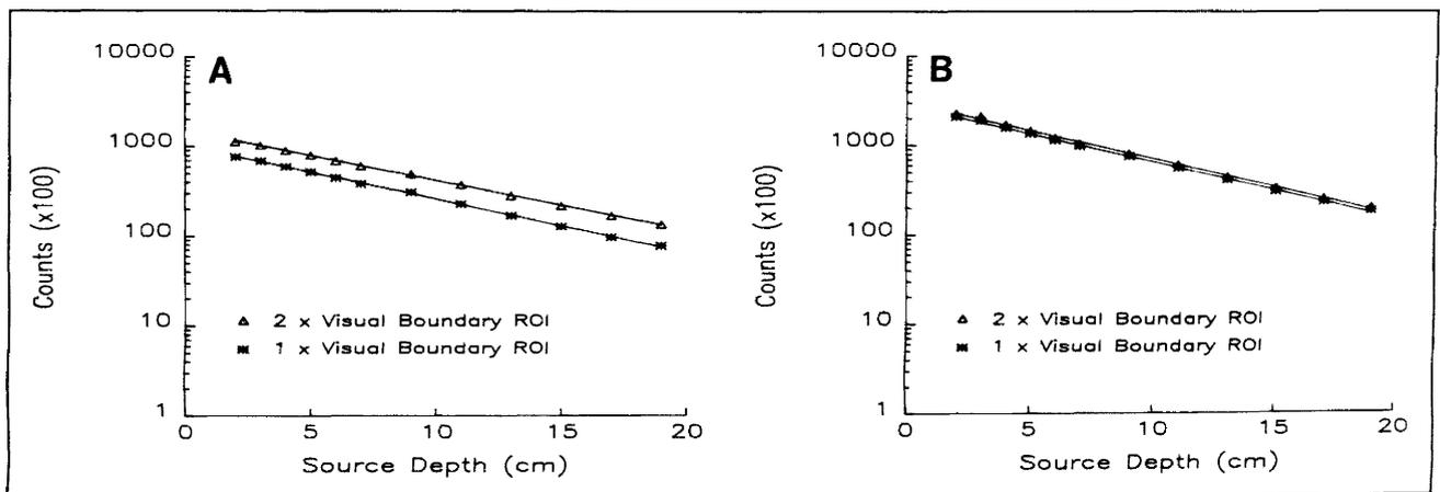
**FIGURE 2.** Linear regression fits to the experimental data from the small spherical source (i.d. = 3.75 cm). (A) Raw data and (B) Wiener filtered data versus source depth in scatter as a function of ROI size. "1 x Visual Boundary ROI" corresponds to ROI1 and "2 x Visual Boundary ROI" corresponds to ROI2.
