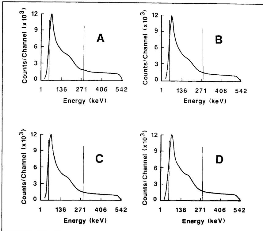
**FIGURE 1.** Bremsstrahlung energy spectra recorded from a point source of  $^{32}\text{P}$  at (A) 5 mm, (B) 50 mm, (C) 100 mm, and (D) 150 mm depth in the scattering medium. The vertical lines indicate the selected energy window.
