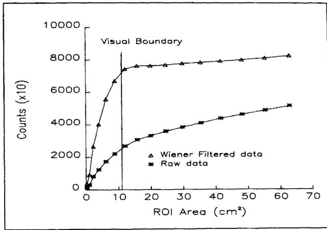
**FIGURE 4.** Plots of ROI counts versus ROI area for the small spherical source (i.d. = 3.75 cm) at a depth of 10 cm in the scattering medium. The visual boundary (ROI1) was, as indicated, essentially the same for the raw and filtered image. The fraction of total photons, however, detected within ROI1 is larger for the filtered image as shown in Table 5.
