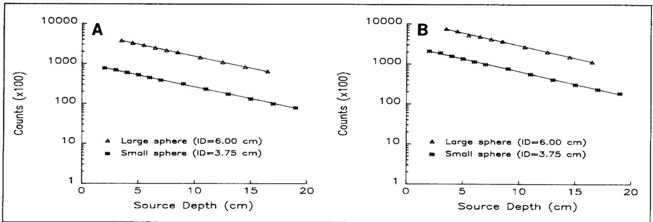
**FIGURE 3.** Linear regression fits to the experimental data from ROI1 of both sources. (A) Raw data and (B) Wiener filtered data versus source depth in scatter as a function of source size.
