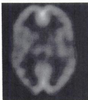
FIGURE 13. Physically measured reconstructed image of a basal ganglia slice within the physical brain phantom imaged with point-focusing collimators.
