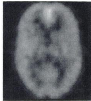
FIGURE 8. Physically measured reconstructed image of a basal ganglia slice within the physical brain phantom imaged with parallel-hole collimators.
