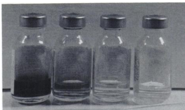
FIGURE 1 Effect of pH and oxygen on the stability of ^{18}\text{F} -6-FD. 6-FD samples from left to right are: (1) pH 7 under ambient air; (2) pH 7 under helium gas; (3) pH 3.5 under helium gas; and (4) pH 3.5 under oxygen gas. Note that samples (3) and (4) are clear, sample (2) is slightly colored, while sample (1) is dark.
